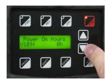
4. Using the arrow key, scroll to parameter V108. This parameter displays the total time that the machine has actually been running.
