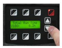
5. To exit the programming menu, simply press the program (PROG) button. This should bring you back to the main operation screen.
