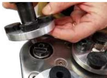
3. Attach the Low Profile Pad Driver, applying a generous amount of blue threadlocker compound (Loctite 243) to the bolt and the threaded drive shaft. Insert the bolt through the hole in the pad driver.
