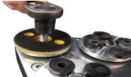
5. Once the bolt is engaged, make sure the drive shaft is properly seated within the pad driver slot before tightening the bolt all the way.
